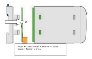
8) After inserting the Back cover transducer, can be used for required application..
