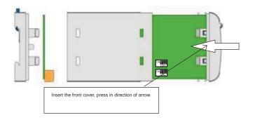
7) After inserting the front cover insert the Interface card PCB and back cover..
