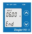
Pressing the " V Down" key will enter the "New/Change End value of Input edit" mode.
