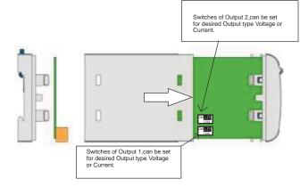
6) After changing the switches for desired Output, Insert the front cover.
