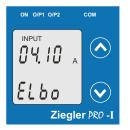
New/changed Elbow value of the Input confirmed.
